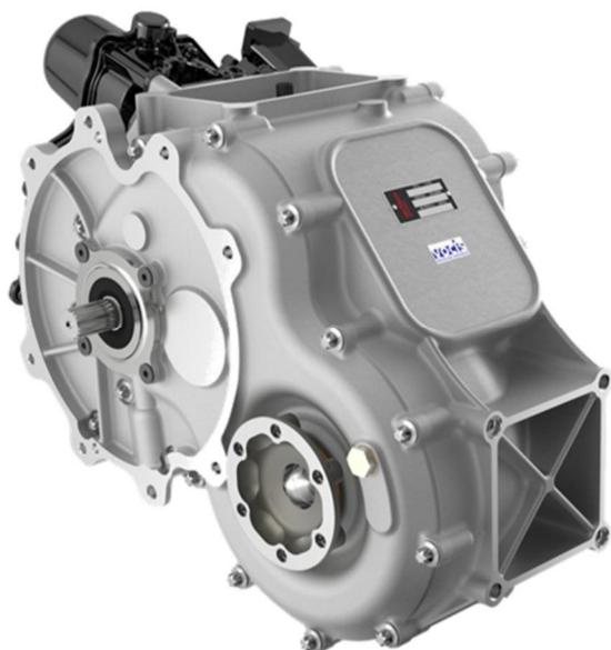
*Figure 2: The first assembled prototype unit, with both motors mounted at the same ends of the transmission*
